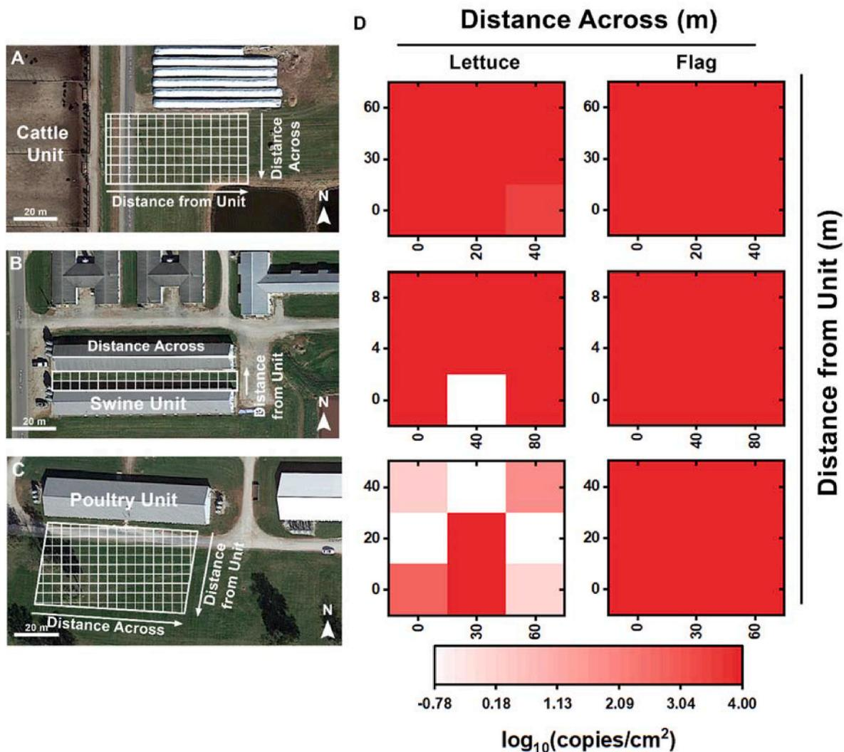
**Fig. 5.** Risk of fecal contamination mapping using LAMP (Universal.Bacteroidales.16s rRNA.1). The Tt value of each LAMP reaction was converted to  $\log_{10}$  (copies/ $\text{cm}^2$ ) via a linear fit to log-transformed concentrations (Fig. S6 A).
